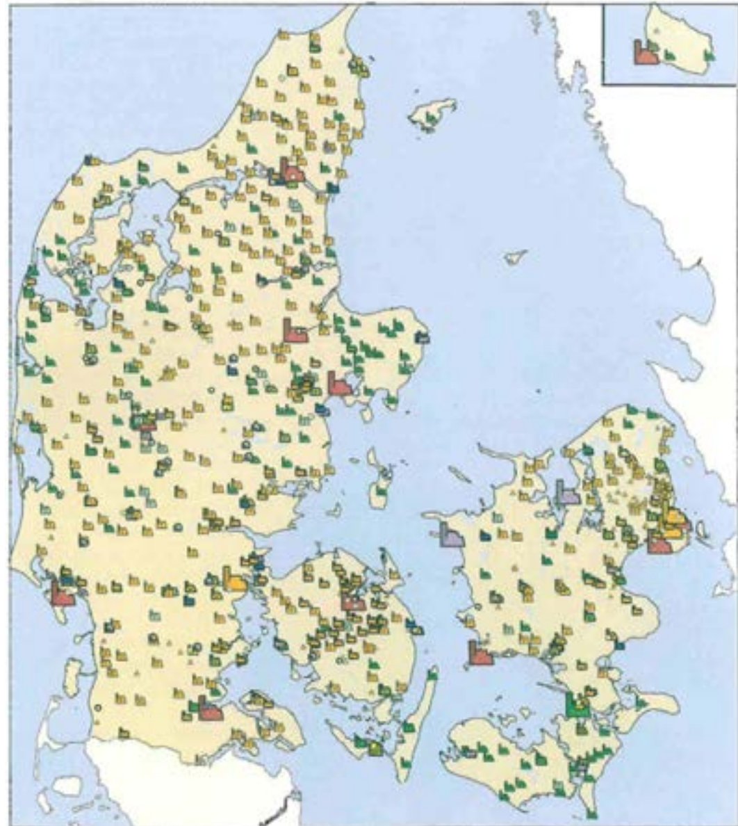
Figure 1. More than 400 DH and CHP plants cover the country of Denmark and the most dominant type by far is the decentralised CHP plant.
